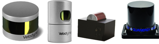
Fig. 4. Lidars with curved reception glasses. Velodyne’s VLP-16, HDL-32E, IBEO’s LUX Mini, and Quanser’s M8 (from left).
