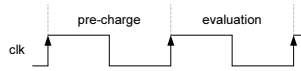
Fig. 10. Sequence of pre-charge and evaluation phases in an MDPL circuit using MDPL D-flip-flops without timing constraints
